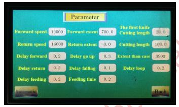
The first knife Cutting Length: Fist cutting length Cutting Length: Cutting length starting from second cut
