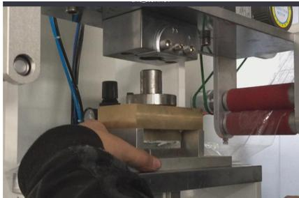
3) Make sure the upper part of the mold is in correct position then screw to fix the upper part of the mold and make sure it is not loose.
