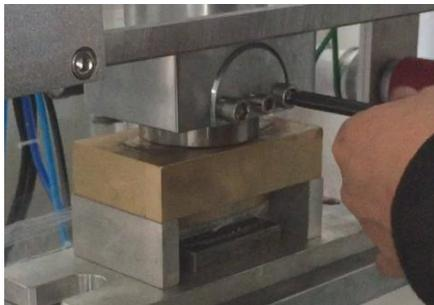
4) Press Manual Up Button and then press the Manual Down button again to double check if the base part of the mold is in correct position, adjust the position of base part of the mold if needed. Check again if the upper part and base part of the mold are perfectly matched, then screw to fix the base part of the mold and make sure it is not loose.
